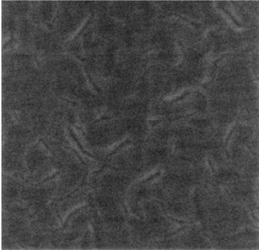
Secondary Electron image of Antiphase domains of GaAs on Ge
